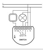
Double switch - mains electricity power connection
