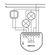
Fig.1 Wiring diagrams for Double Relay Switch.
