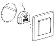
Fig.2 Installation of Fibaro Relay Switch in wall switch box
